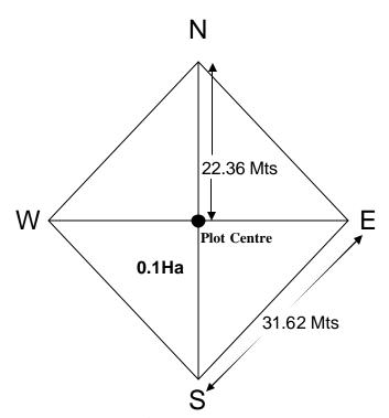
After fixing the plot centre fix the N, S, E and W corners of the plot by measuring 22.36 m, horizontal distance by tape/rope in all four directions. Stout pegs or bamboo of 1.5 m height should be fixed at each corner and a flag attached to it. Check the correctness of layout by measuring each side, which should be 31.62 m.
